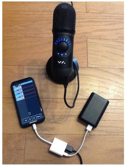
Note that the battery may also be plugged directly into Spatial Mic, however plugging the battery into the Adapter as shown will also charge the mobile device.
