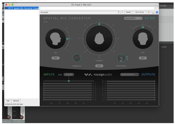
13. Next, click **Add** and insert the **FB360 Converter plugin** (<u>available for download here</u>). To listen to mic playback in binaural stereo, setup plugin as shown (note that after closing and reopening a session, check to make sure the correct output is still selected
